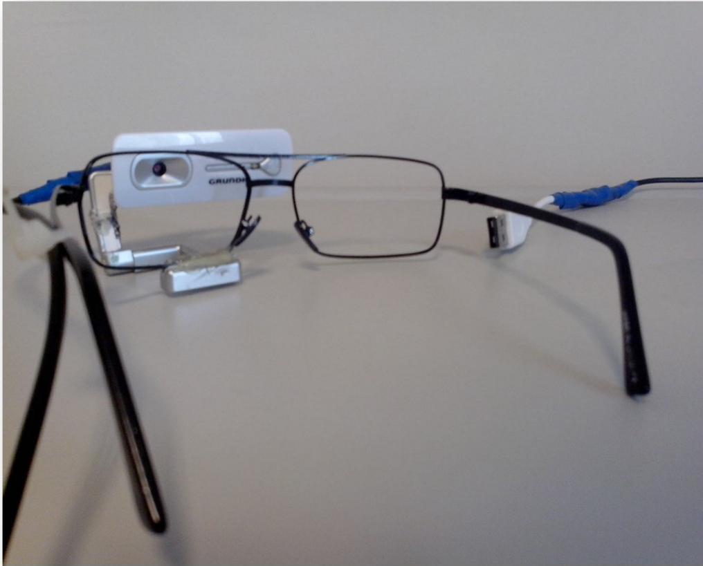
Figure 8: The Final Appearance of the eye-tracking device
