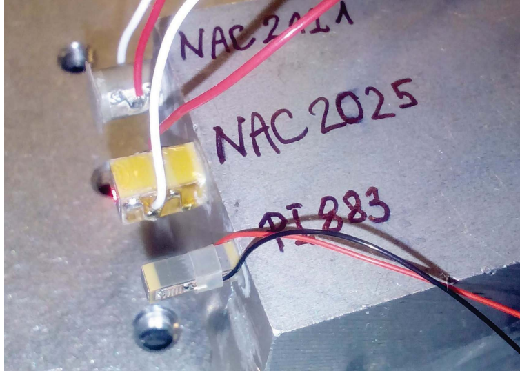
Figure 2.3: Stacked piezo actuators of different manufacturers prepared for characterization by a vibrometer
