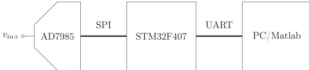
Figure 2.7: Data acquisition system consisting of an ADC (AD7895) which digitizes the analogue signals, a real time processing system (STM32F407) which executes filtering algorithms and a PC with data evaluation in MATLAB.
