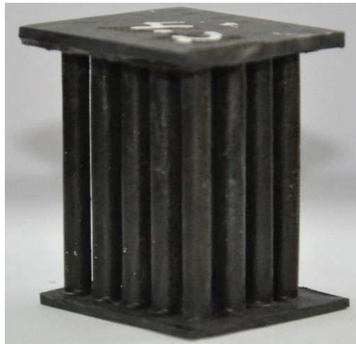
Figure 5.3: The unit cell of a column truss core based on an array of 4 mm diameter columns.
