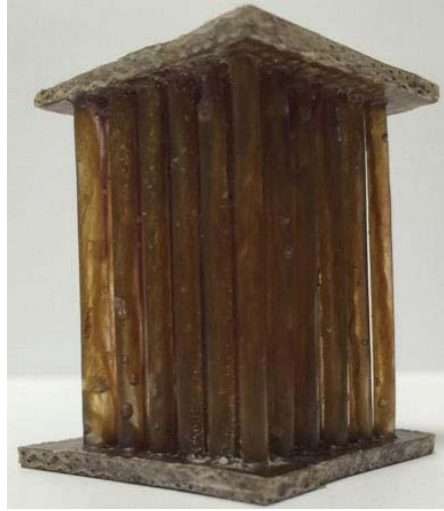
Figure 5.4: Photograph of a 6 x 6 column core based on 2.5 mm diameter struts.
