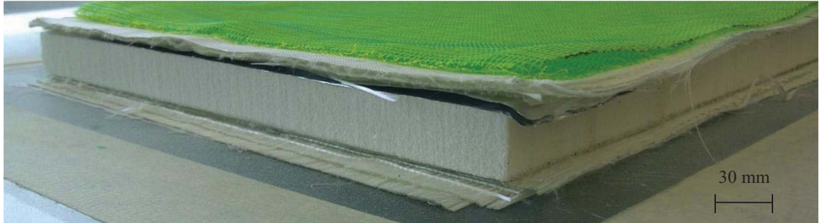
Figure 2.12: Stacking procedure completed in preparation for vacuum bagging and infusion.
