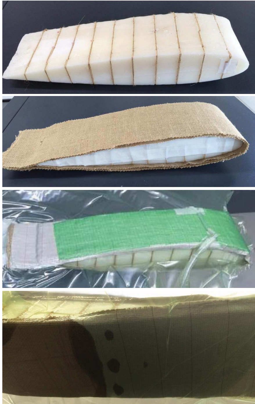
Figure C.1: Photographs showing (a) Jute fibers passing through the holes in the wax mold in a continuous fashion, (b) Natural fiber sheets forming the airofoil skin placed around the mold, (c) airofoil stack sealed in a vacuum bag in preparation for the infusion process (d) and flow front on one side of the airfoil during the VARTM process.
