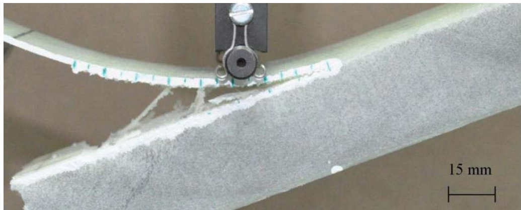
Figure 5.41: Photograph of the edge of Material F-D during interfacial fracture testing.
