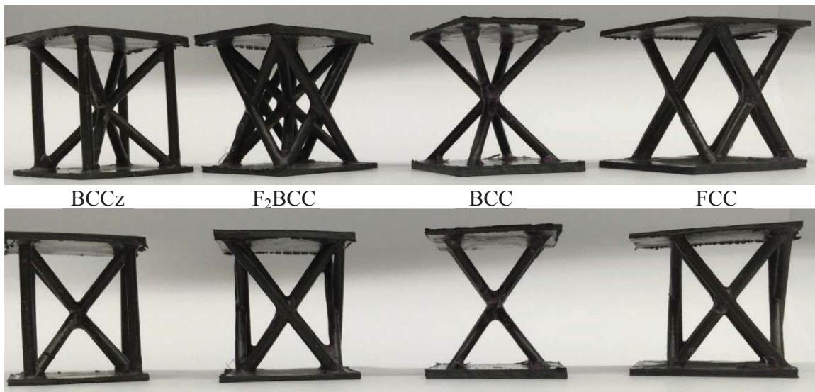
Figure 5.8. Photographs of the BCCz, the F 2 BCC, the BCC and FCC lattice structures following manufacture.
