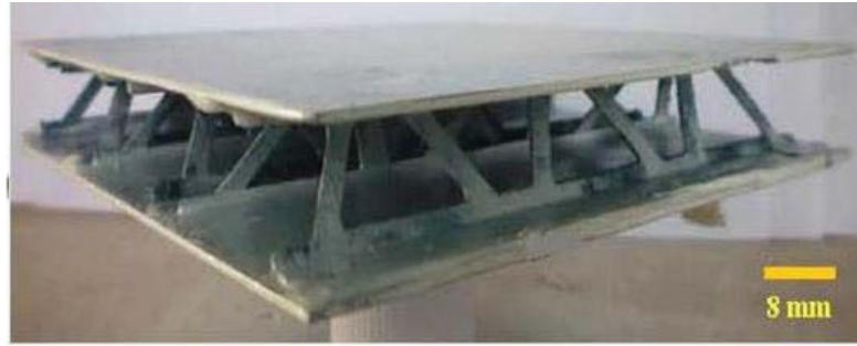
Figure 1.24: EDM Pyramidal carbon fiber reinforced epoxy lattices having a core relative density of 4.95% [34].
